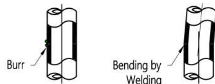
[Fig. 3-4] Wrong Pipe-Welding Connection
